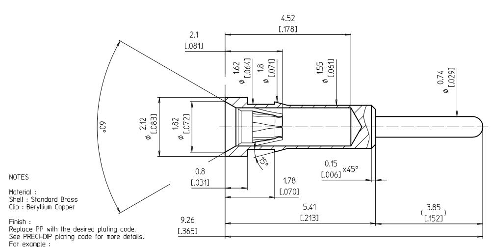
Replace PP by 83 for Tin on the barrel and 0.75µm gold on the Clip. See the availability of plating configuration on preci-dip website
