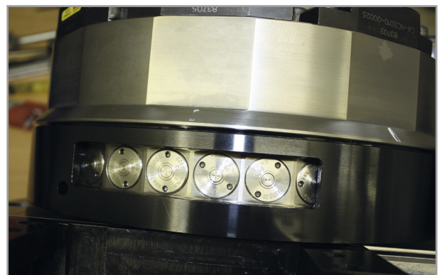
The revolver with a total of 36 coupling nipples.
